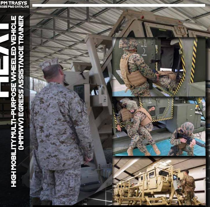
The High Mobility Multi-Purpose Wheeled Vehicle Egress Assistance Trainer (HEAT) provides a realistic and relevant training environment for Marines to train tactical vehicle egress procedures in various degrees of vehicle rollover. Marines experience the real effects of a vehicle rollover, practice egress through cab doors and turret opening, receive reinforcement of the importance of wearing a seat belt and learn the procedures and effort levels required to execute vehicle egress.
