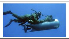
**Overview:** The Diver Propulsion Device (DPD) is part of the Amphibious Reconnaissance program. It is an underwater motorized device that provides a range up to 3.5 nautical mile (NM) underwater delivery of a combatant dive pair to conduct amphibious reconnaissance missions in support of the Marine Air-Ground Task Force (MAGTF). The DPD improves diver range, payload and speed.
