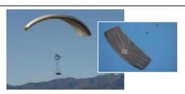
**Overview:** The Joint Precision Airdrop System 10,000 lbs. (JPADS 10K) is a precision airdrop system with an autonomous guidance unit for controlled flight upon release from the aircraft and provides reduced ground load dispersion through superior landing accuracy.
