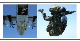
Overview: The Tandem Offset Resupply Delivery System (TORDS) system allows a parachutist to deliver heavy loads (equipment or personnel) in conjunction with military free-fall operations, increasing the payload of required combat essential equipment.
